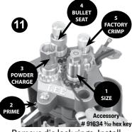
Remove die lock rings. Install dies according to instructions. IMPORTANT Lee die set users,
