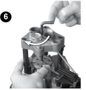
Raise carrier to the mid-stroke position, install shell plate, lightly tighten clockwise with 1/4" hex head wrench
