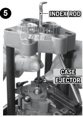
Remove index rod and case ejector.
