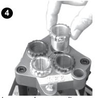
Loosen and remove spline drive breech lock bushing to access index rod.
