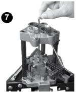
With the carrier near the bottom of the stroke (handle up), install index rod.
