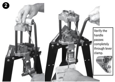
Re-position handle, tighten securely with 1/2" wrench.
