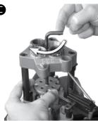
Raise carrier to the mid-stroke position, install shell plate, lightly tighten clockwise with ¼" hex head wrench.
