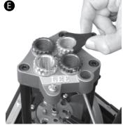
Install Spline Drive breech lock bushing.
