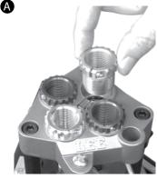
Remove Spline Drive breech lock bushing.
