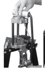
Verify the handle passes completely through lever clamp.
