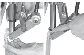
Raise ram to mid-stroke position. Install primer arm in the carrier.
