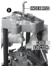
Remove index rod and case ejector.
