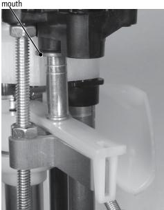
C The 4 tube feed plate should be a penny's thickness away from the tool head casting. Verify a coins thickness away from body.
