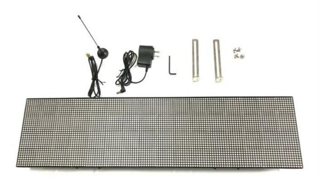
3. If you purchased M1A2-W shot timer and LED display in the same order, please install the antenna to led display first. Plug in the power and turn on the LED display first and then turn on shot timer. After that, they will get connected automatically.
