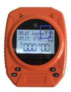
C. Turn on the shot timer--Settings--System--RFID--Timer, please change the timer's RF channel to the same as LED display, then reboot the shot timer and you can see they get connected successfully.
