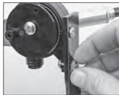
Insert (2) 8-32 x 1/2" screws (FT1940) through body and steel stand and tighten with (2) nuts (FE3364)
