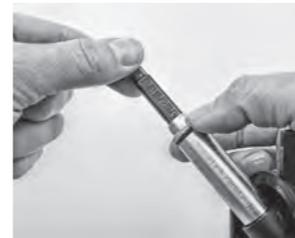
■ Turn the thimble to the number 3 on the metering rod for the whole number to the left of the decimal point. The #3 indicator line must be visible when the thimble is at zero.
