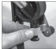
Insert drop tube into body; screw knurled nut (AP1640) tight to body.
